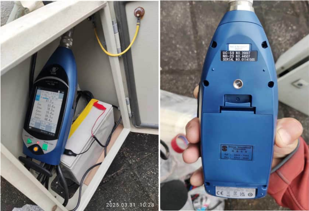
Noise monitoring equipment at NM2
